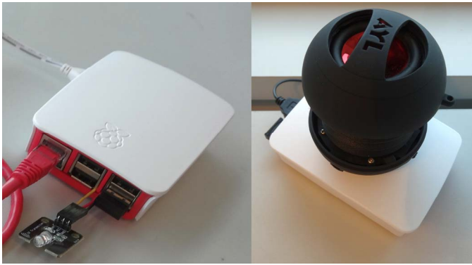
Fig. 4. Raspberry Pi with an infrared emitter (left). Raspberry Pi with an USB audio speaker (right).
